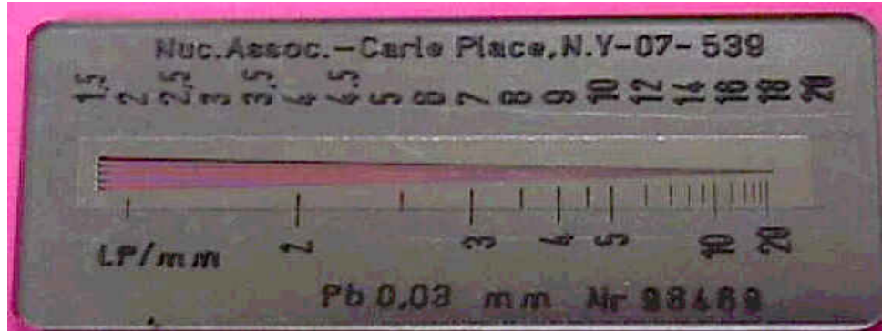
Figure . Photograph of line pair gauge made by Victoreen.
